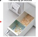
Remaining kernels and crushed kernels are separated into different travs.
